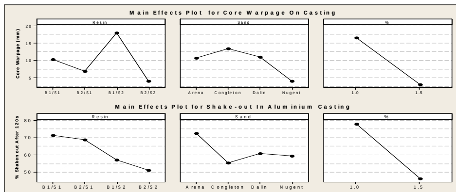
Figure 8: Core warpage on casting and shake-out performance.
